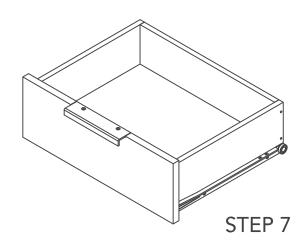
Attach Drawer Front (G1) and Drawer Back (G2) to Drawer Side (G3) with 1 1/4" Flat Head Screws.
