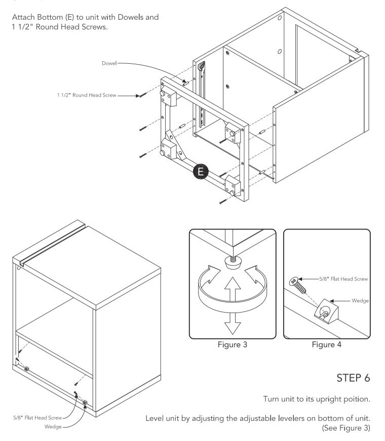
Attach Wedges to unit with 5/8" Flat Head Screws. (See Figure 4)
