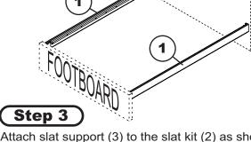
Attach slat support (3) to the slat kit (2) as shown below using JCB M6 X 25mm (B) and cap nut (C). Tighten with Allen wrench (E).
