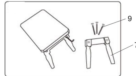
Make sure the barrel nuts trip are lined up with the holes. Then attach the legs with the screws and use the allen wrench to tighten the barrel nuts.
