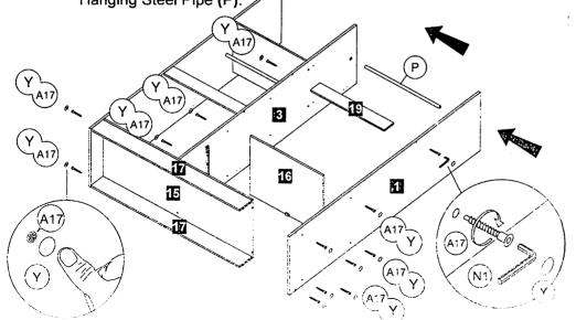
STEP 7 Insert the Hanging Steel Pipe (P). Use Allen Key (N1) to tighten the Crosshead Screw m6.3 x 40mm (17) & button the screw head with Crosshead Cover (Y) except crosshead screw at panel no. 15.
