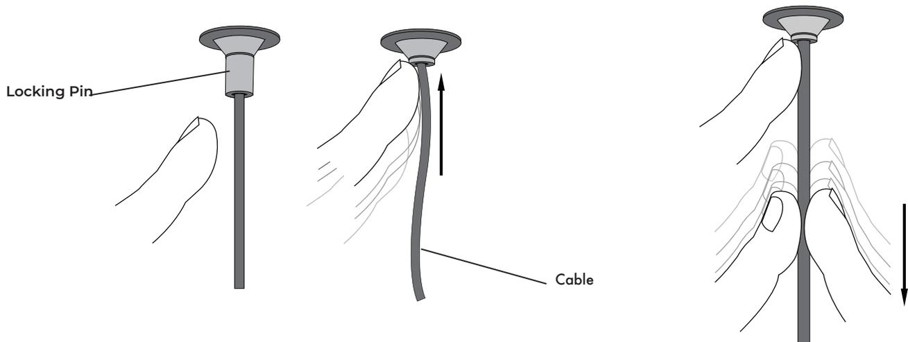
The length of the cable is adjustable. To determine the proper length of the fixture, hold the fixture canopy up against the outlet box in the ceiling to adjust the cable.
