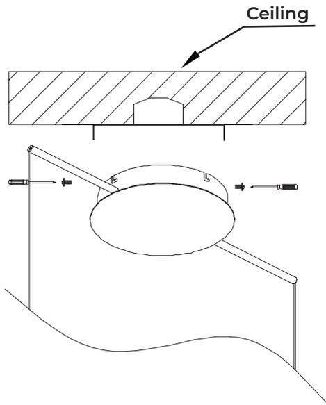
Secure canopy to mounting bracket (A) with canopy screws (G).
