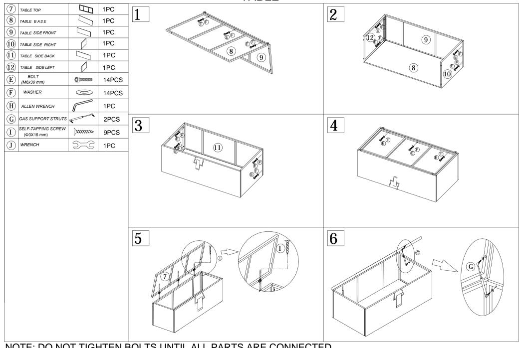
NOTE: DO NOT TIGHTEN BOLTS UNTIL ALL PARTS ARE CONNECTED YOU MAY FIND CUSHIONS PLACED UNDERNEATH THE TABLE AND STORAGE BOX OR BETWEEN FRAMES!
