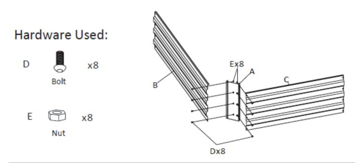
② Do the same way to other 3 frames and panels. Tighten bolts and nuts with Allen key (F).
