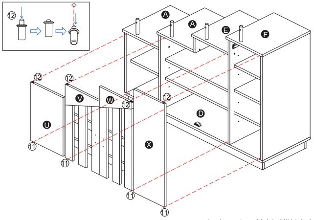
Insert non-spring assisted pin (#11) into the hole of the unit first before the spring assisted pin (#12).
