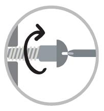
Turn clockwise to tighten and only tighten when step is completed or when instructed to do so.
