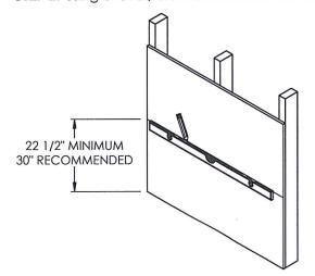
**STEP 3.** Attach the wall cleat (6) with notch facing the wall, using six modz screws (H) and using the line (step2) to make sure it is level.
