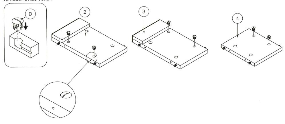
STEP3. POSITION LEFT SIDE PANEL (2) AND RIGHT SIDE PANEL (3) TO THE EDGES OF THE TOP (1) [DETAIL A 1) POSITION CENTER DIVIDER (4) TO CENTER OF THE TOP (1)
