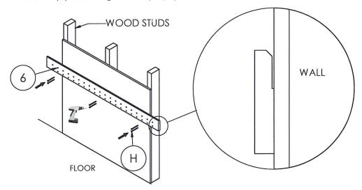
**STEP 4.** Mounting the console requires two people, carefully lower the console brackets (B) onto the wall cleat (6) until the unit fits tightly into the wall cleat.
