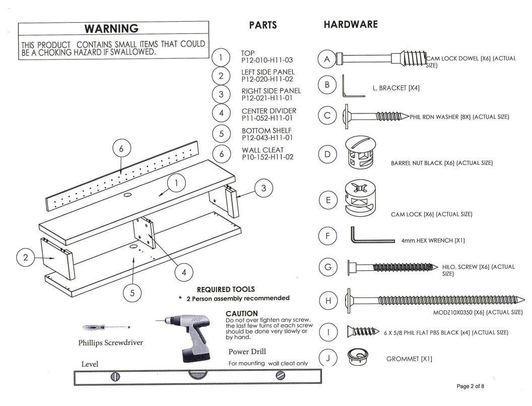
**STEP 1.** INSTALL SIX CAM LOCK DOWELS (A) INTO TOP (1). INSTALL FOUR L-BRACKETS (B) INTO THE LOCATOR HOLES ON THE TOP (1) USING EIGHT PHILLIPS WASHER SCREWS (C).
