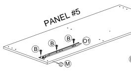
Using a hammer gently tap the 3 Plastic Pin M into the bottom edge of Panel #2, & 5.
