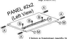
Using a hammer gently tap the 3 Plastic Pin M into the bottom edge of Panel #9, 11 & 13.
