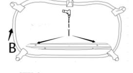
STEP 2 Please screw off the bolts from the wood frame underneath the loveseat with electric drill.
