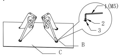
Place the Table top (C) on the Table top frame (B)by screw (M8\*12mm)
