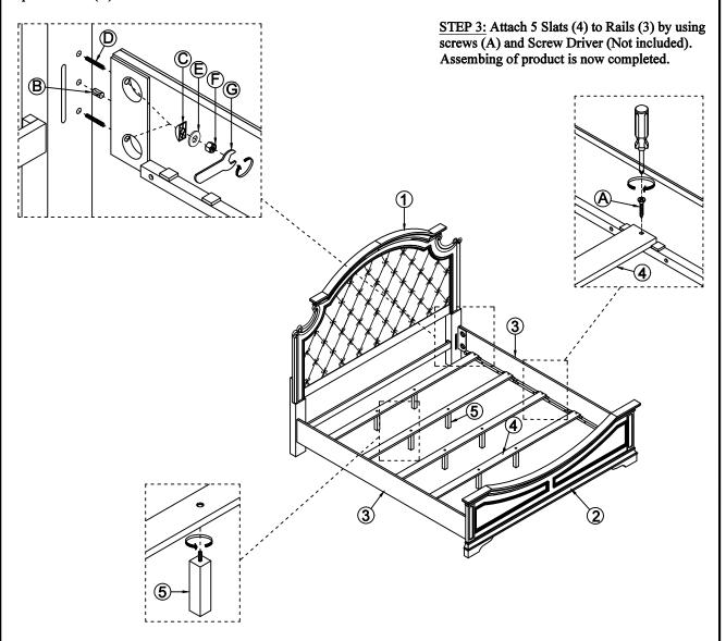
STEP 2: Securing 10 Supports Leg (5) into 5 Slats (4).
