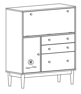
To move door left or right, loosen screw as shown and move door to suit. Re-tighten screw.
