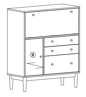
To move door in or out, loosen screw as shown and move door to suit. Re-tighten screw.
