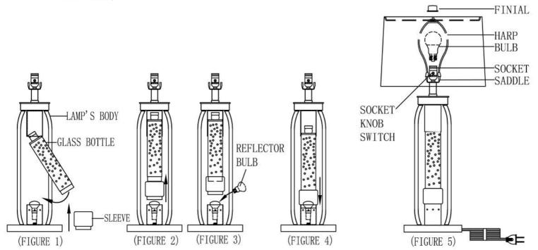
IF THE REFLECTOR BULB IS BURNT OUT AND REQUIRES REPLACEMENT, PLEASE TURN OFF THE POWER AND WAIT UNTIL THE LAMP COOL DOWN ENTIRELY, THEN FOLLOWING THE STEPS.
