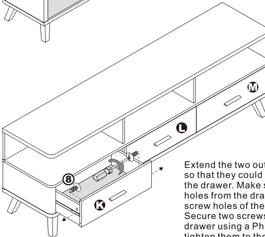
Extend the two outer slides of the runners so that they could align with the sides of the drawer. Make sure the pre-drilled holes from the drawer align with the screw holes of the outer slides. Secure two screws from the inside of the drawer using a Phillips screwdriver to tighten them to the outer slides.
