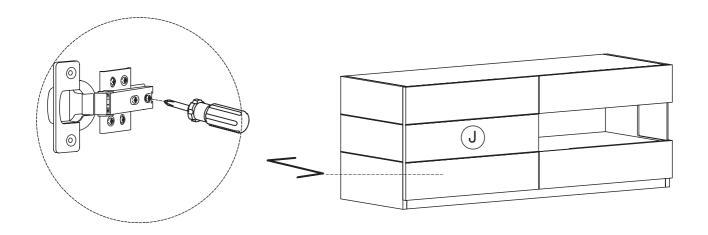
To move door in or out, loosen screw as shown and move door to suit. Re-tighten screw.
