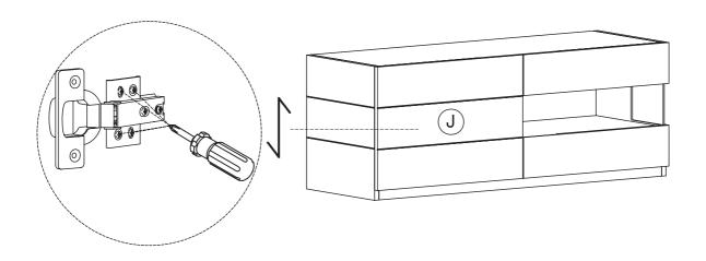
To move door up or down, loosen screws as shown and move door to suit. Re-tighten screws.
