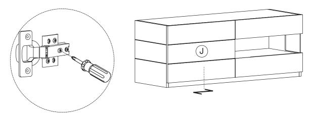
To move door left or right, loosen screw as shown and move door to suit. Re-tighten screw.
