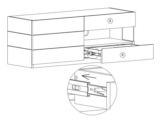
Line up the drawer glides on the drawers on both sides so that they enter evenly into the extended receiving side panel drawer glides as shown then gently push in the drawer until the drawer is secure and slides in and out smoothly.
