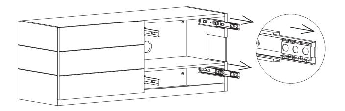
Slide out the side panel drawer glides for proper insertion of the drawers.
