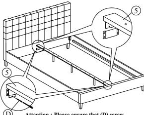
Attention: Please ensure that (D) screw is being attach as per the A.I shown to avoid base being collapse.
