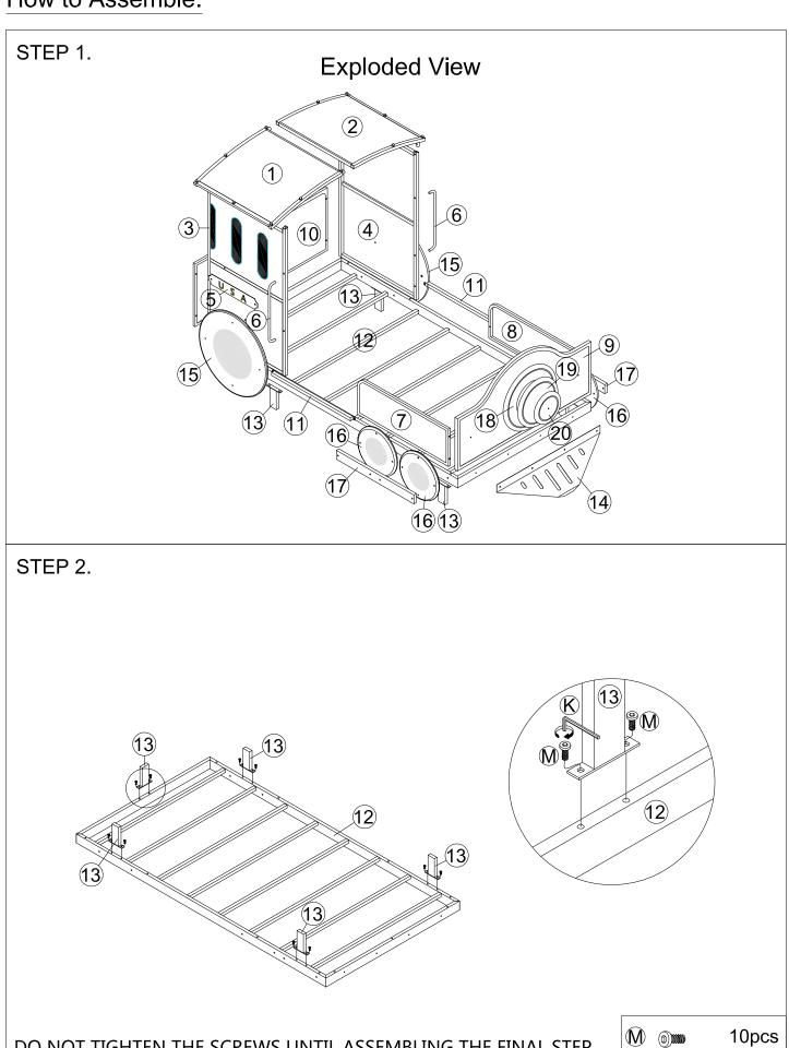
DO NOT TIGHTEN THE SCREWS UNTIL ASSEMBLING THE FINAL STEP.
