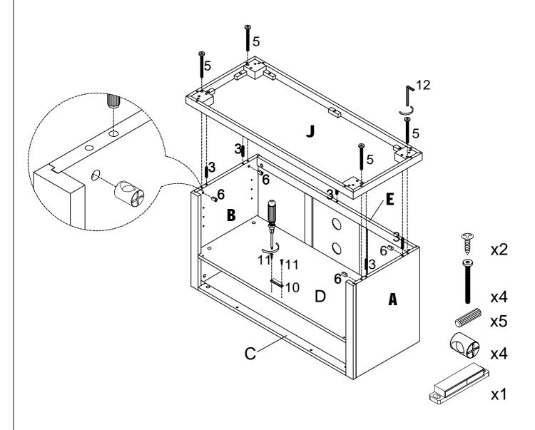
Step 8. Attach Top I to cabinet using Wood Dowels & Cam locks as shown. Secure Rail C to Top I using Screws (Part #4) through pre-drilled holes as shown.
