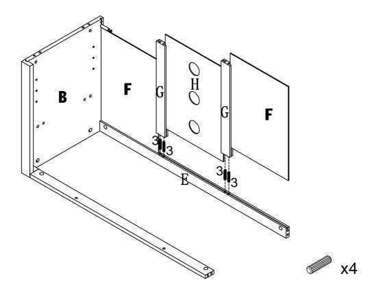
Step 4. Insert Wood dowels into the top end of rails G. Attach rail E to Panel B & Rails G using Wood dowels & Cam locks as shown.
