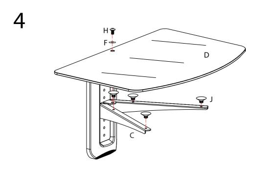
Insert rubber pad(J) into the holes of metal support(C), put glass shelf(D) onto rubber pad, then fix it with screw(H) and washer(F).
