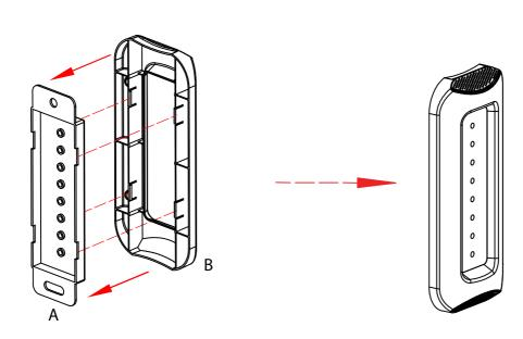
Attaching cover(B) to wall plate(A).
