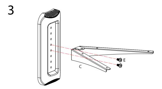
Attaching metal support(C) to wall plate(A) with screws(E) and allen wrench(K) according to your desired height.
