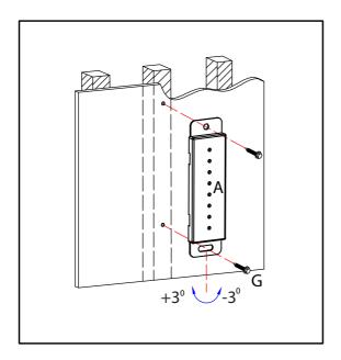
This shelf is designed to be mounted into wood studs.
