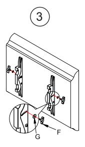
3.Attach the handles(F) to the mounts through washers(G).
