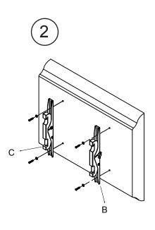
Attach TV mounts(B&C) to the back panel of TV. Make sure you choose the same height of screw holes in TV mounts.
