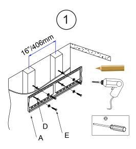
1.Hold wall plate(A) against wall at desired position, then using a pencil mark 4 hole locations. Then drill holes according pencil marks using 5/16" or 8mm size drill bit to a depth of 2.5"/64mm.
