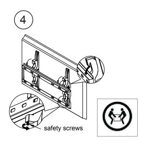
4. Hang up the TV to wall plate, then fix the safety screws tightly.
