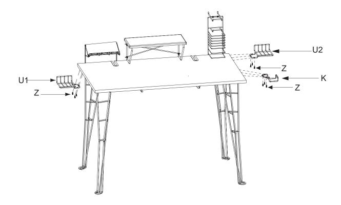
4.Fix the speaker tray (U1 & U2) to the top panel with screws (Z),fix the headphone holder (K) with screws (Z).
