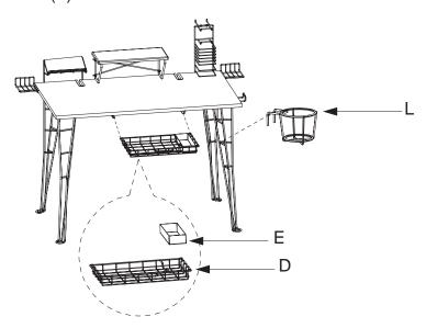
5. Fold the plastic sheet (E) to rectangular shape, then put it into drawer (D), insert the drawer into the rail, hang the cup hold (L) to the leg.
