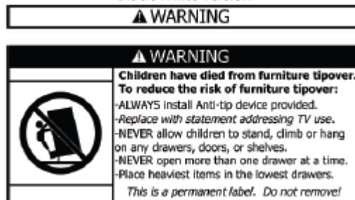
Figure 2. Example warning For Clothing Storage units that are designed and intended by the manufacturer to be used with a TV.
