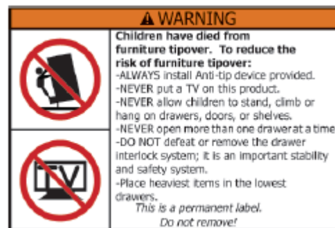
Figure 3. Example warning for unit with Interlocks Not Designed and Intended by the Manufacturer to be Used with a TV.
