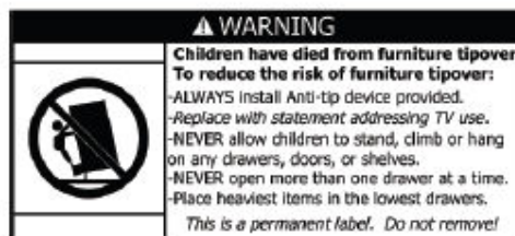
Figure 2. Example warning For Clothing Storage units that are designed and intended by the manufacturer to be used with a TV.
