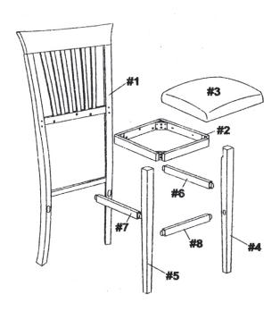
For ease of identification all parts are labeled to correspond to the Step number in which the part is used.
