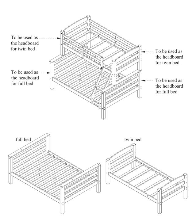
To convert the bunk bed into a full size bed and a twin bed, remove the ladder and all the guardrails. With the help of another person, remove the top bunk from the lower bunk.
